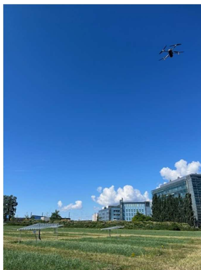
Figure 4. Drought measurements on the biodiversity test field from an UAV platform.
